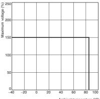
Ambient temperature (°C) Note: "Maximum voltage" is the maximum voltage that can be applied to the Relay coil. Shock Malfunction
