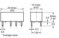
Note: Each value has a tolerance of ±0.3 mm.
