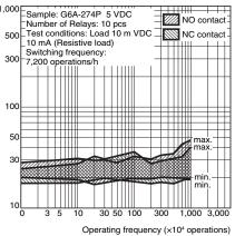
The tests were conducted at an ambient temperature of 23°C. \*1. \*2. The contact resistance data are periodically measured reference values and are not values from each monitoring operation. Contact resistance values will vary according to the switching frequency and operating environment, so be sure to check operation under the actual operating conditions before use.
