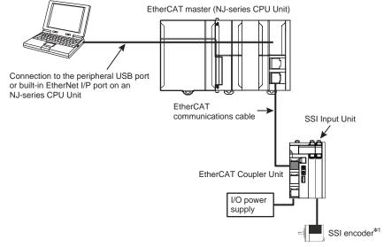
\*1. The SSI encoder is supplied with 24-VDC power from the SSI Input Unit.
